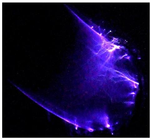
Intense sparking observed at the edge of lamination (sharp corners intensify electric field)
