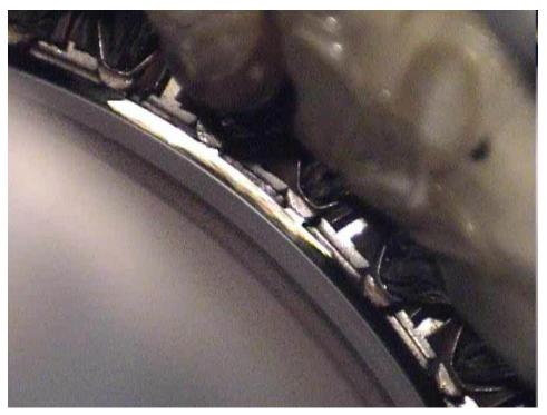
Rotor bars can be swaged for a tight fit in the slot. Photograph courtesy of Notified Body
