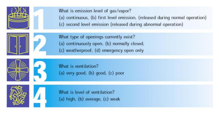
Basic approach: Reduce to an acceptable level the probability of coincidence of a flammable atmosphere and a source of ignition
