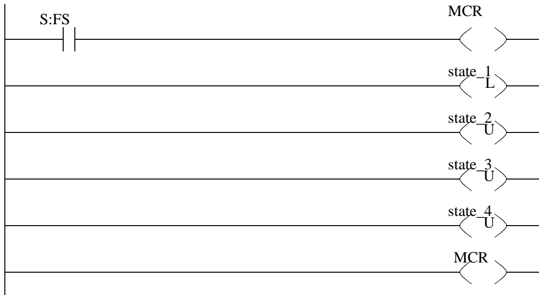
Figure 22.10 Ladder Logic to Initialize Traffic Light Controller
