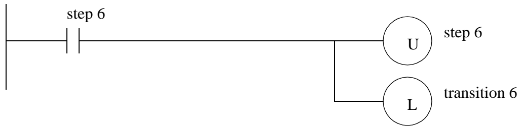
Figure 16.9 SFC Implemented in Ladder Logic
