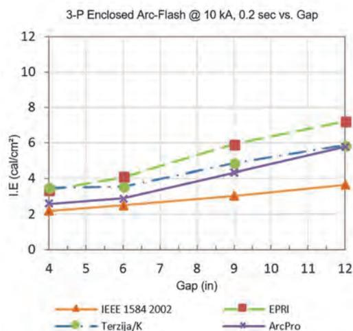
**Figure 6:** 3-P Enclosed I.E. Comparisons for Four Methods
