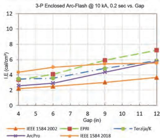
**Figure 7:** 3-P Enclosed I.E. Comparison including IEEE 1584-2018
