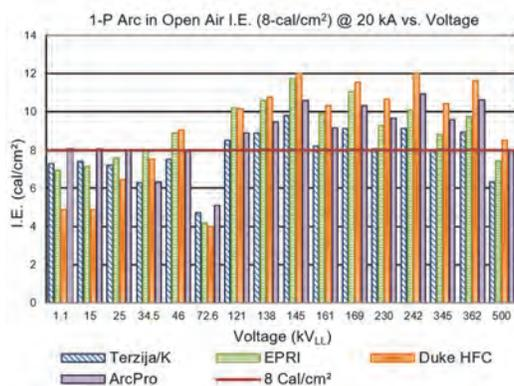
**Figure 5:** Comparison of Four 1-P Arc I.E. Methods – 8 cal
