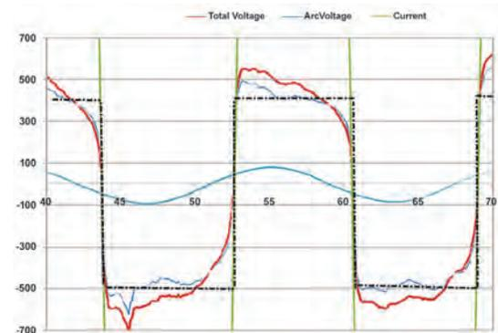
**Figure 2:** Total  $V$  (red),  $V_{arc}$  (blue), and  $I_{arc}$  (green) Waveforms
