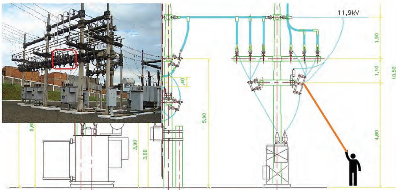
**Figure 3:** *Outdoor Substation*
