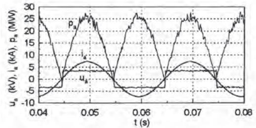
**Figure 1:**  $V_{arc}$  ( $U_a$ ),  $I_{arc}$  ( $i_a$ ), and  $P_{arc}$  ( $P_a$ ) Waveforms
