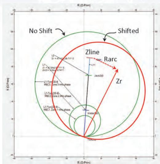
**Figure 1:** Distance Relay Mho Zone Shift for Arc Resistance
