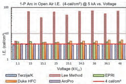
**Figure 3:** Comparison of Five 1-P Arc I.E. Methods – 4 cal
