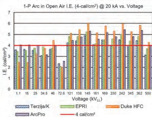
**Figure 4:** Comparison of Four 1-P Arc I.E. Methods – 4 cal
