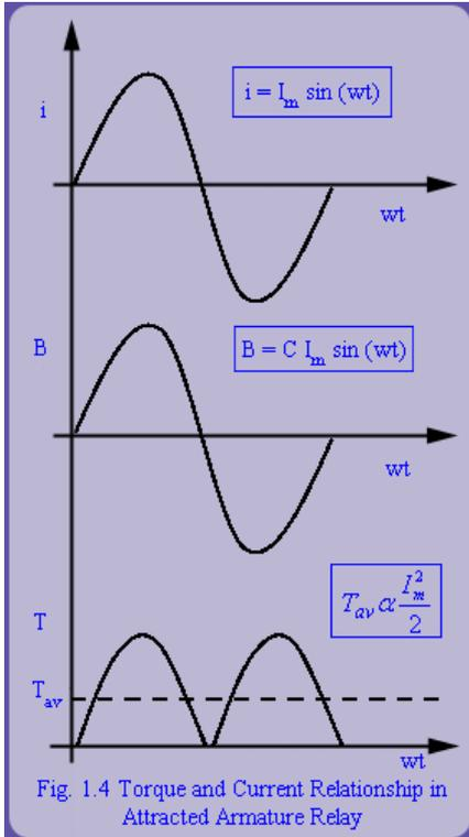
Fig. 1.4 Torque and Current Relationship in Attracted Armature Relay
