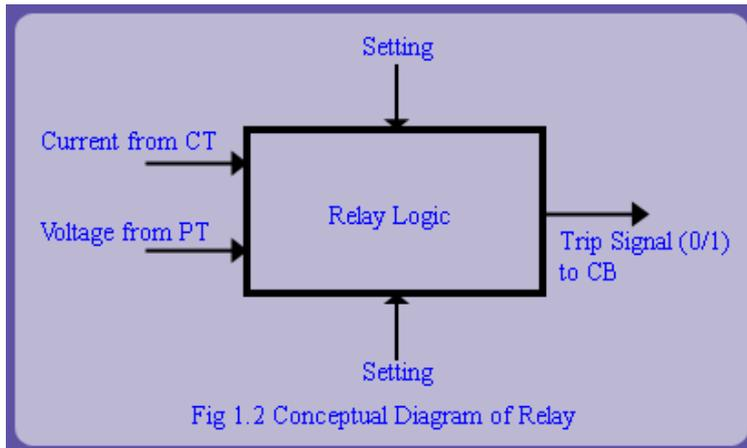
Formally, a relay is a logical element which processes the inputs (mostly voltages and currents) from the system/apparatus and issues a trip decision if a fault within the relay's jurisdiction is detected. A conceptual diagram of relay is shown in fig 1.2.
