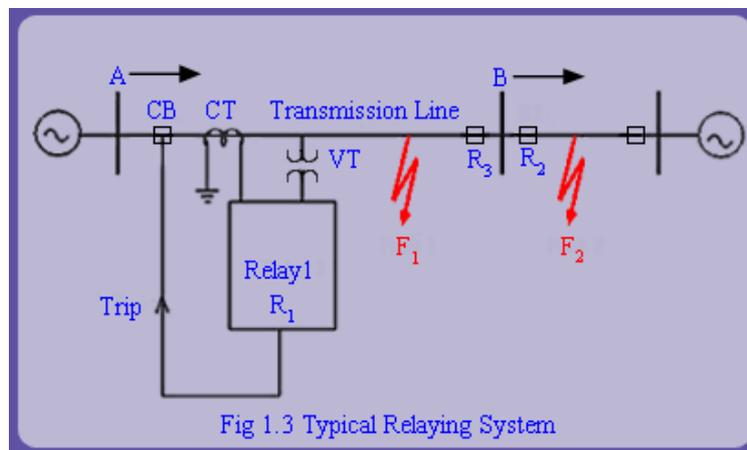
In fig 1.3, a relay  $R_1$  is used to protect the transmission line under fault  $F_1$ . An identical system is connected at the other end of the transmission line relay  $R_3$  to open circuit from the other ends as well.
