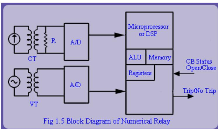
Fig 1.5 Block Diagram of Numerical Relay
