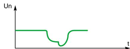
**Fig. 7** : main types of interruptions and voltage dips.
