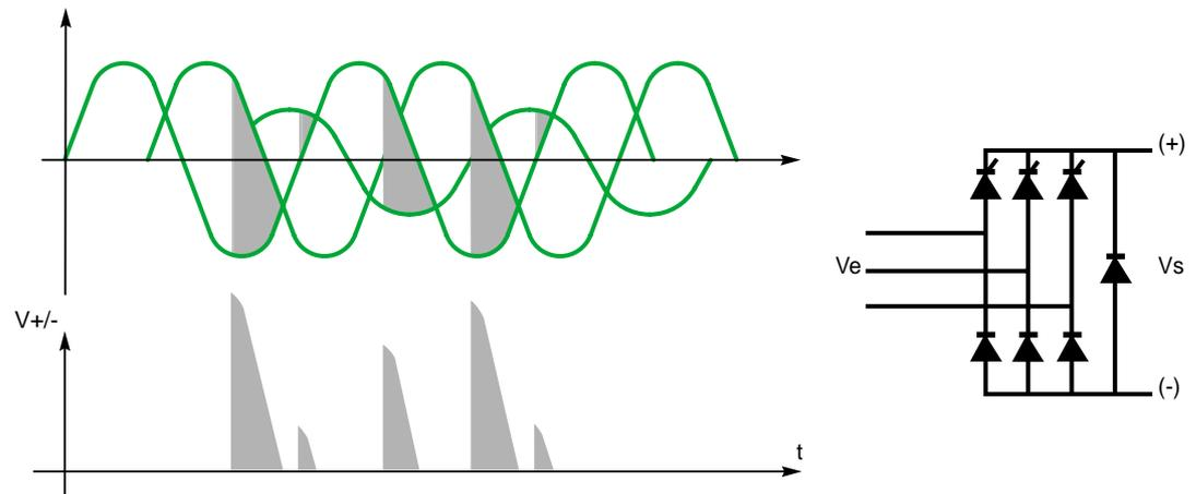
**Fig. 30** : effect of a voltage unbalance on a rectifier in semi-controlled Graetz bridge.
