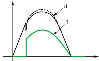
**Fig. 27** : voltage and current waves distorted by a heating dimmer.
