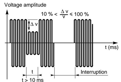
**Fig. 1** : voltage dip ( $\Delta v$ ) and interruption.
