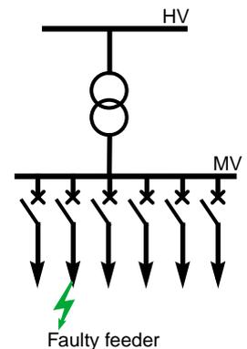
**Principle:** On an overhead MV network, most faults are intermittent. Thus, the incoming circuit-breaker on each feeder is equipped with an automated system that attempts two reclosings (sometimes three):
