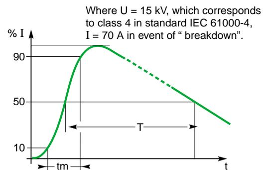
**Fig. 35** : electrostatic discharge current (tm = 5 ns, T = 30 ms).
