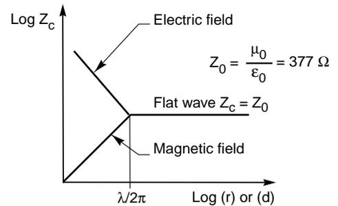
Fig. 33 : example of wave impedance for a bipole.
