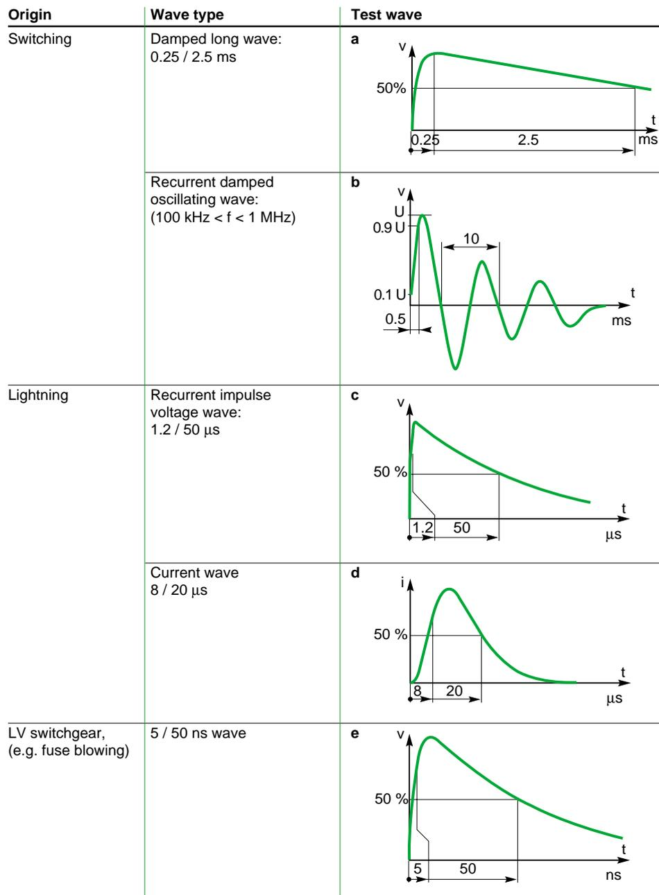
**Fig. 21** : the main standardised test waveforms.
