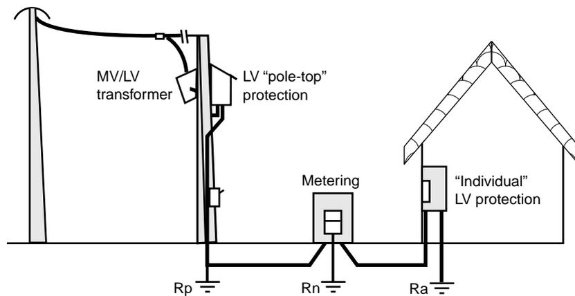
**Fig. 13** : MV/LV “pole-top” substation. TTS earthing system of a MV/LV substation (separate earthing of the spark-gap, transformer frame and LV neutral). This earthing system is ITS if a surge limiter is inserted in the LV neutral earthing connection.
