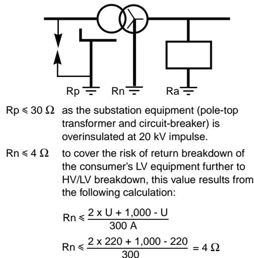
**Fig. 14** : earthing connections of a MV/LV substation supplied by overhead lines.
