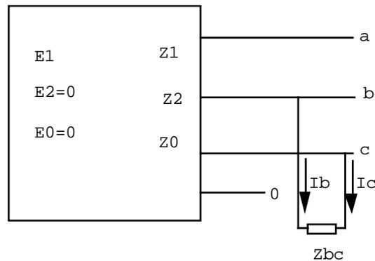
When the impedance “ $Z_{bc}$ ” is inserted, an unsymmetrical current is drawn from the network. The following equations are achieved according to the general, special and basic equations showed above.
