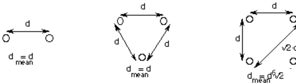
Figure 1. Different conductor configurations.
