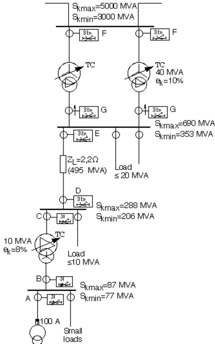
Figure 23. The selectivity plan must cover setting of all the protection relays in the network.
