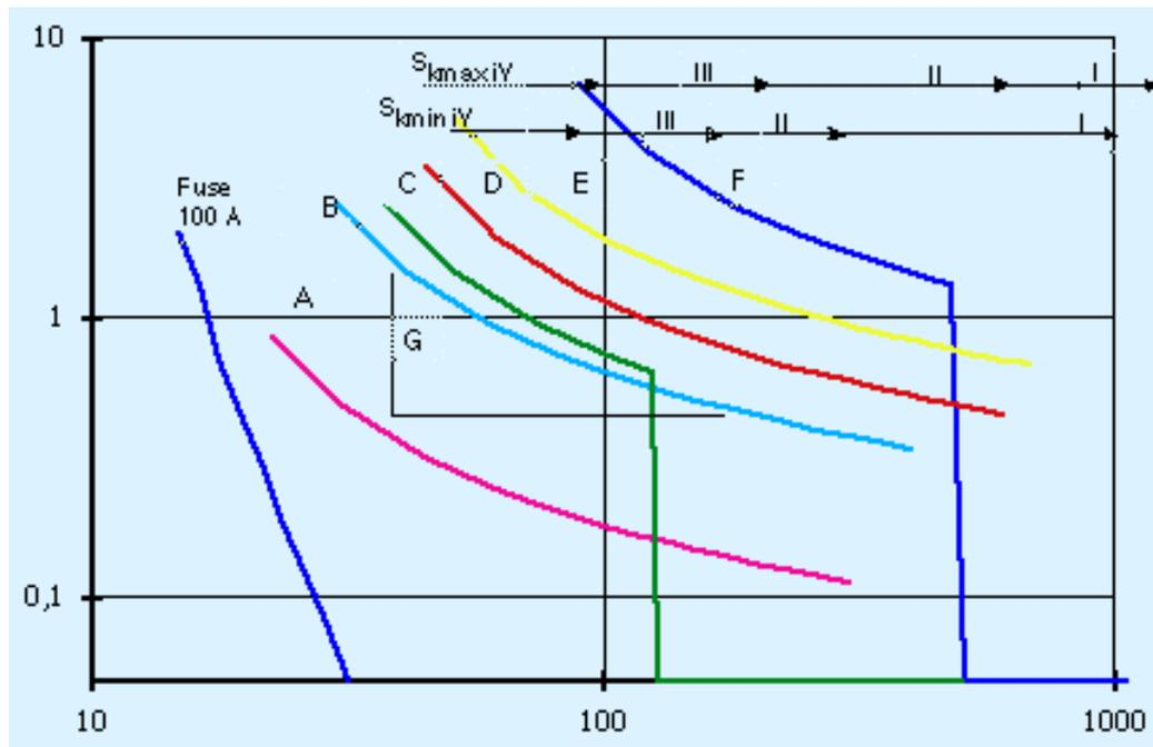
Figure 24. The selectivity plan will have all relays in the network indicated and the time margin must be checked for all selective relays. The sensitivity for back-up protection to fulfil tripping criteria must also be checked.
