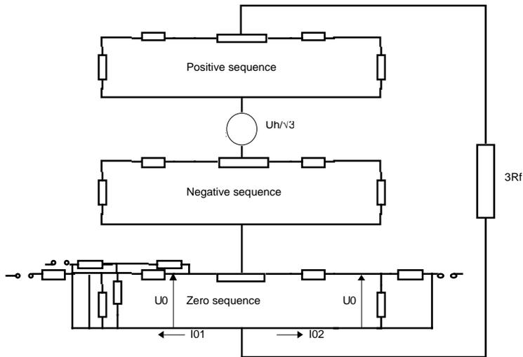
Figure 2. The symmetrical components are used to calculate the “ $I_0$ ” current for the fault in figure 1, “ $3I_0$ ” is the total fault current.
