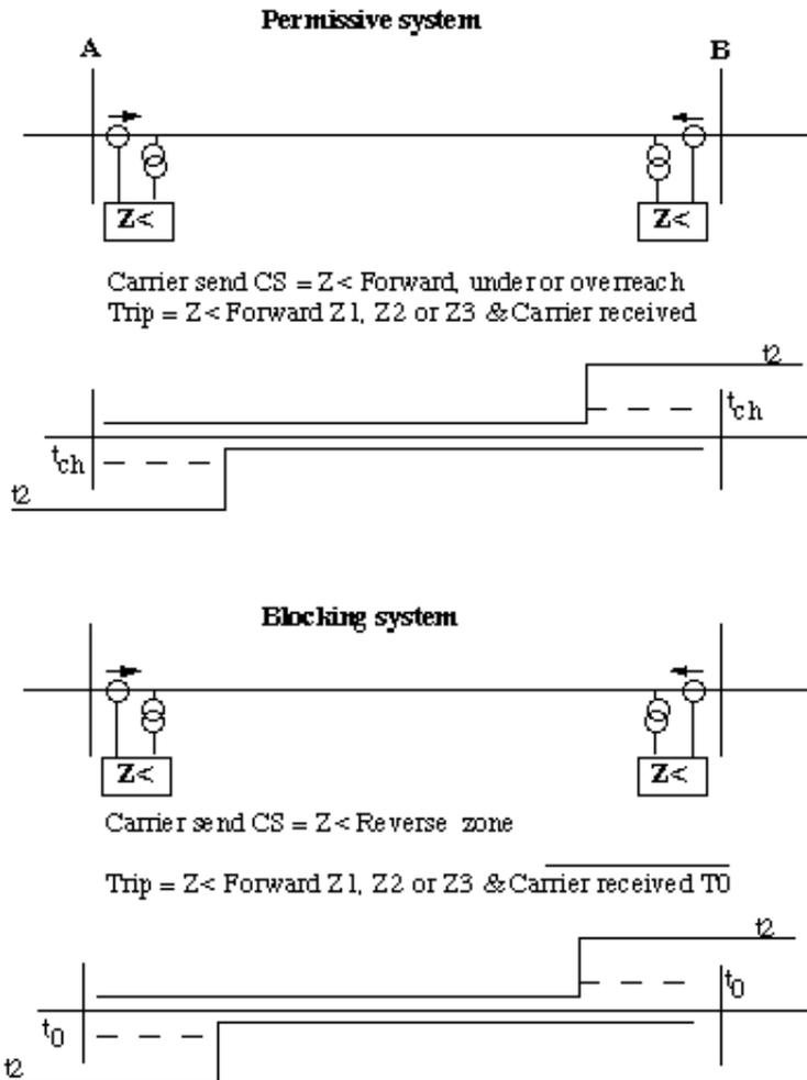
Figure 2. The principle for Distance protection relays communication.
