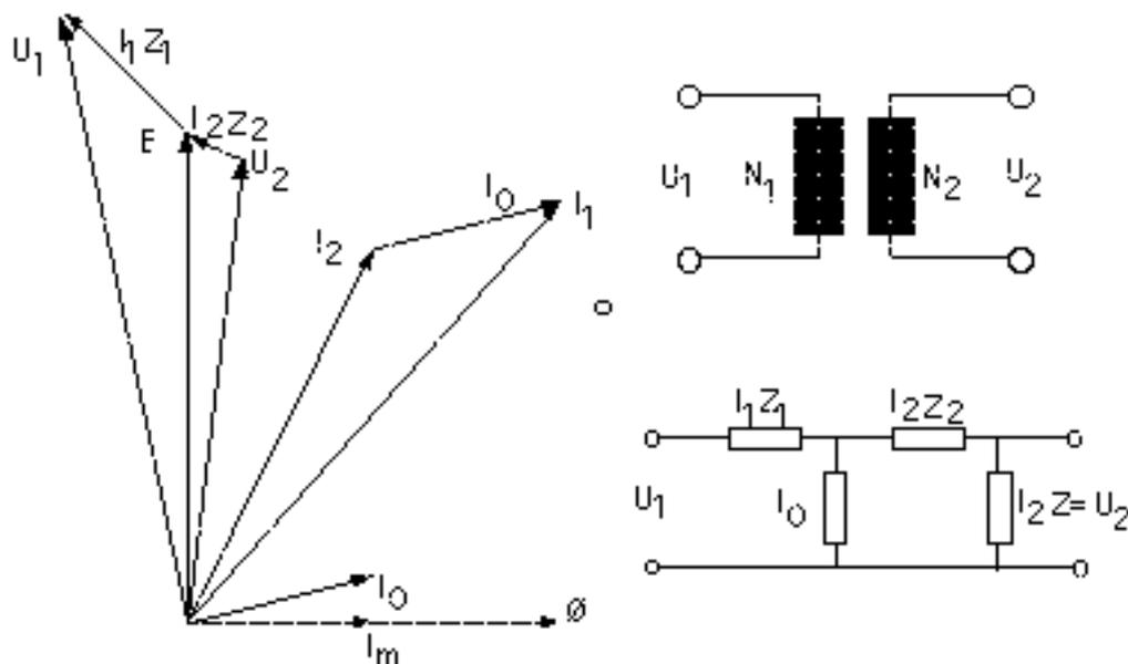
Figure 1. The principle of an Instrument transformer.
