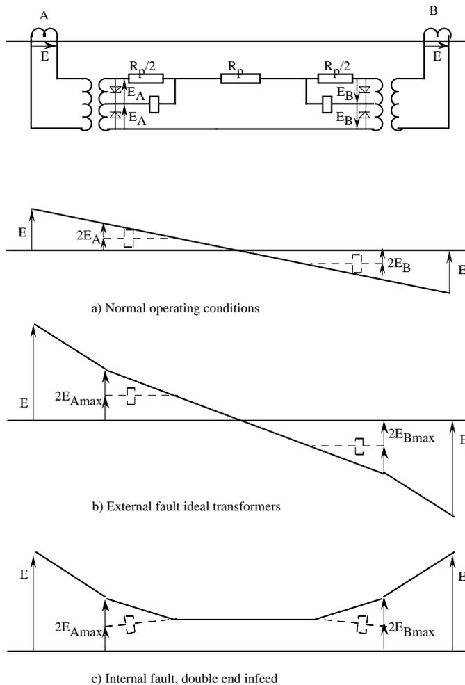
Figure 3. A voltage balance current differential relay
