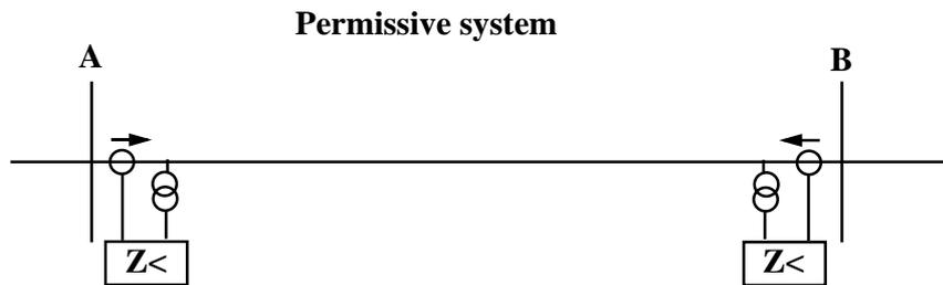
**Carrier send CS = Z< Forward, under or overreach**
