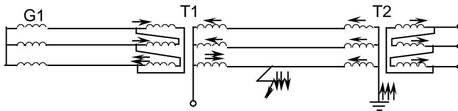
Figure 9. Current distribution in a transmission network.
