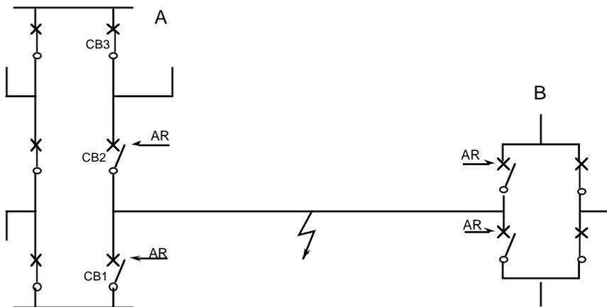
Figure 24. Auto reclosing of transmission line CB:s.
