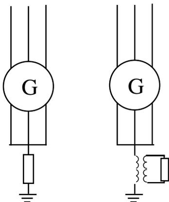
Figure 5. Two equivalent methods for high resistance earthing.
