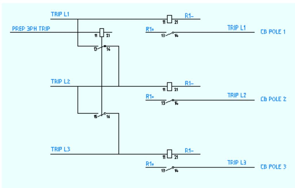
Figure 26. The principle circuit for arrangement of prepare three phase trip at a multi breaker arrangement.
