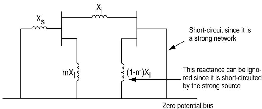
Figure 7. Thevenin's theorem applied on the faulty network.
