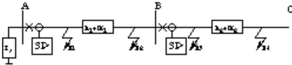
Figure 9. Current selective relays at A and B.
