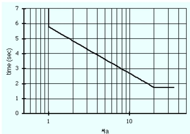
Figure 6. The logarithmic inverse characteristic. A fault current of the biggest infeed less than 0,8 times the current of the faulty object, gives a selective tripping.
