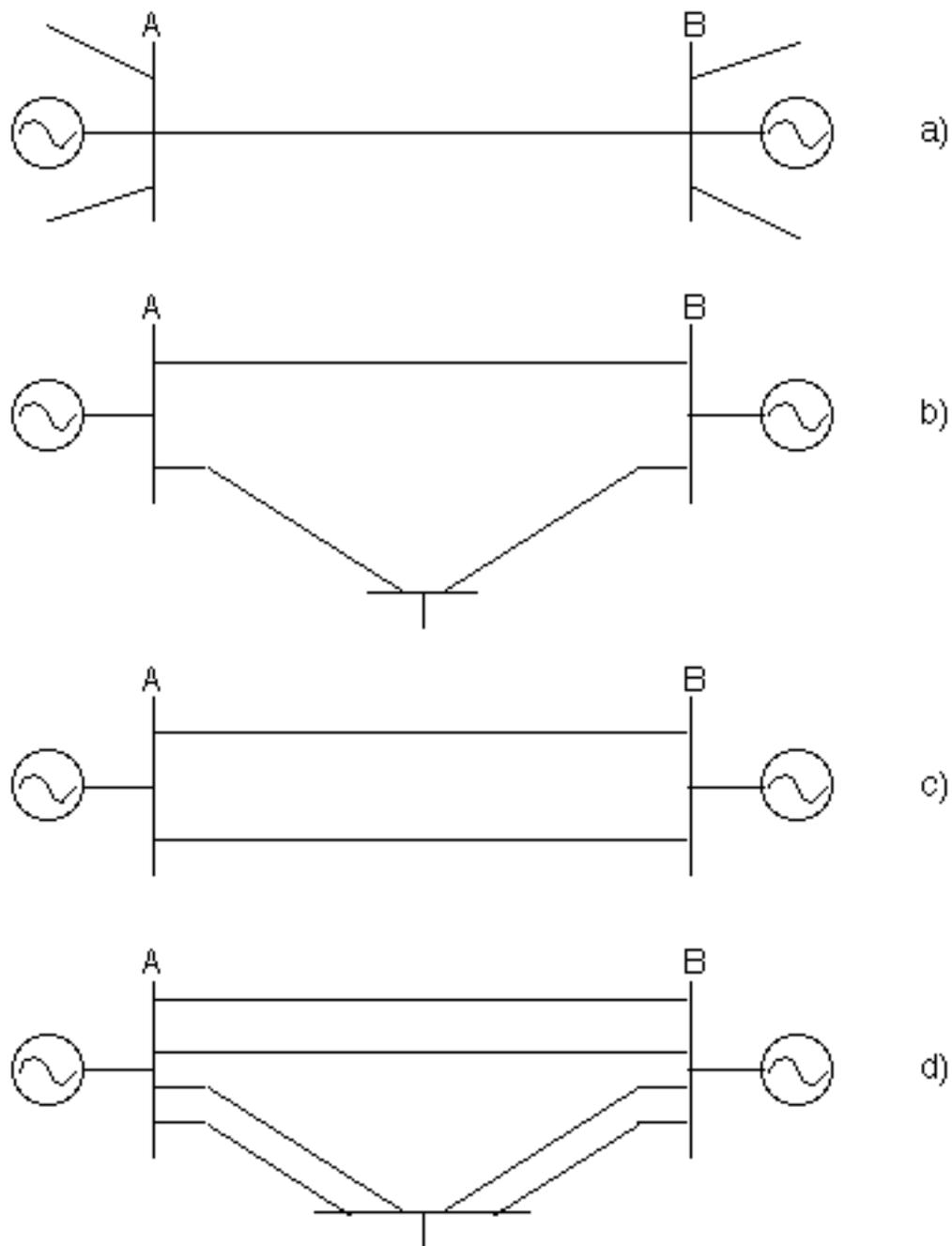
Figure 29. Power grid with different degree of meshing between A and B
