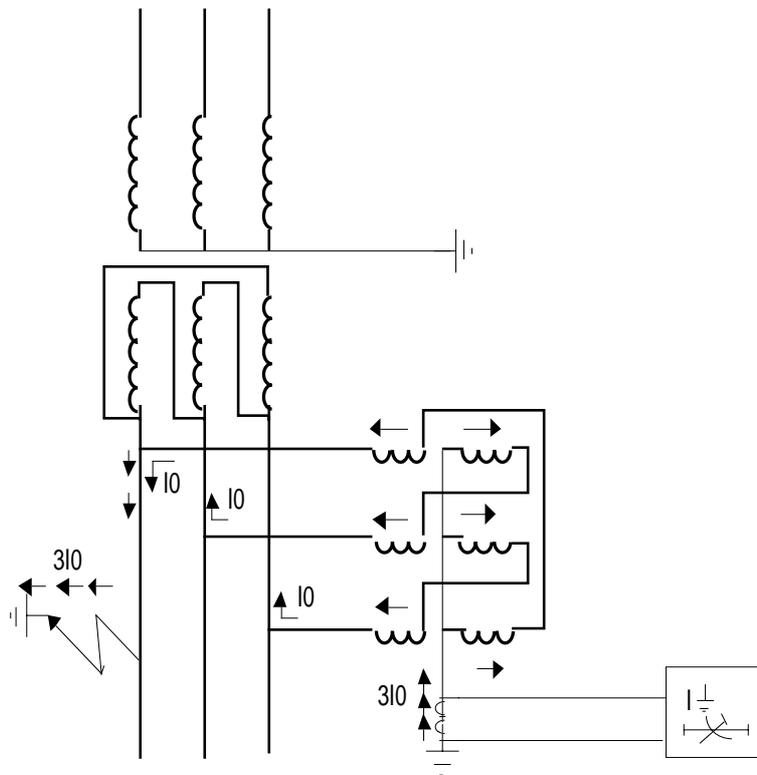
Figure 13. An earth fault protection system for a reactance earthed network where selectivity is achieved by inverse time delayed relays.
