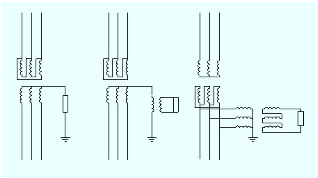
Figure 4. Three equal methods to prevent ferro resonance.
