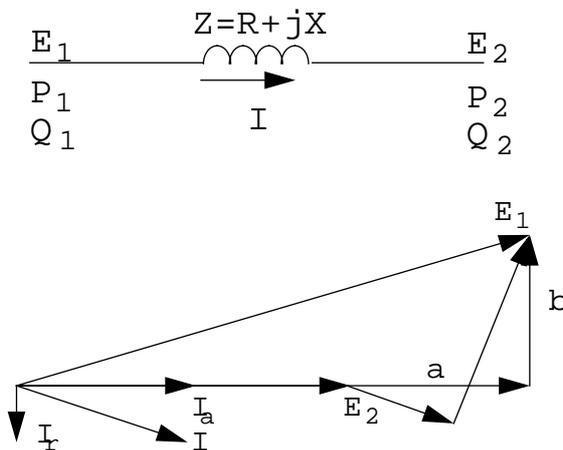
Figure 3. Load transfer on a short line.
