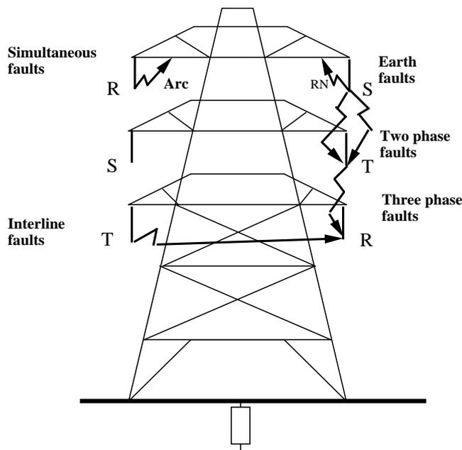
Figure 1. Faults occurring on a transmission line tower are of different types.
