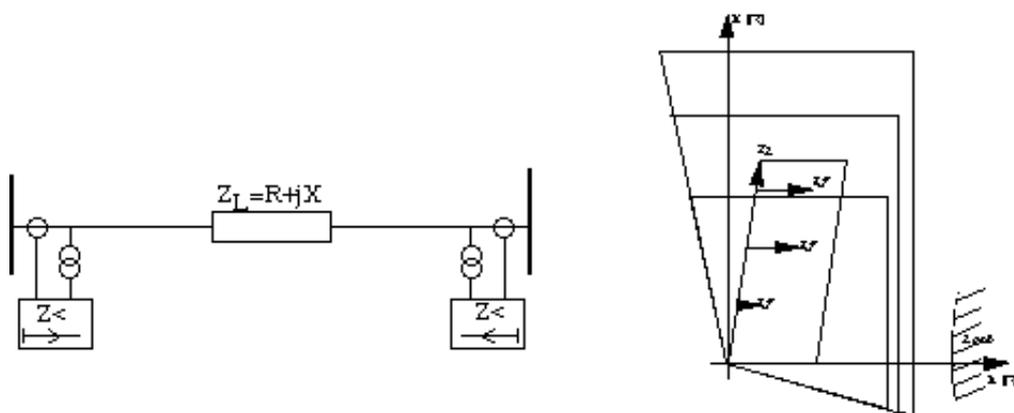
Figure 1. A Distance protection with impedance characteristic for a power line.
