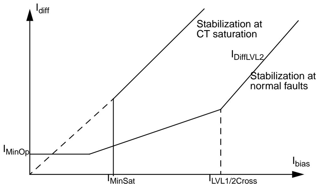
Figure 5. The stabilization characteristic.
