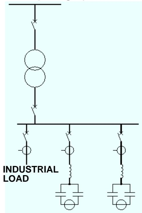
Figure 1. Capacitor banks with series reactors.
