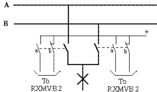
Figure 5. Requirements and connection of busbar disconnector auxiliary contacts, for switching of RXMVB 2 repeat relays.
