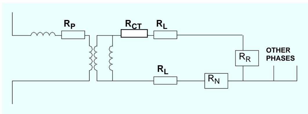
Figure 1. The current transformer principle circuit with magnetizing reactance and secondary resistance.
