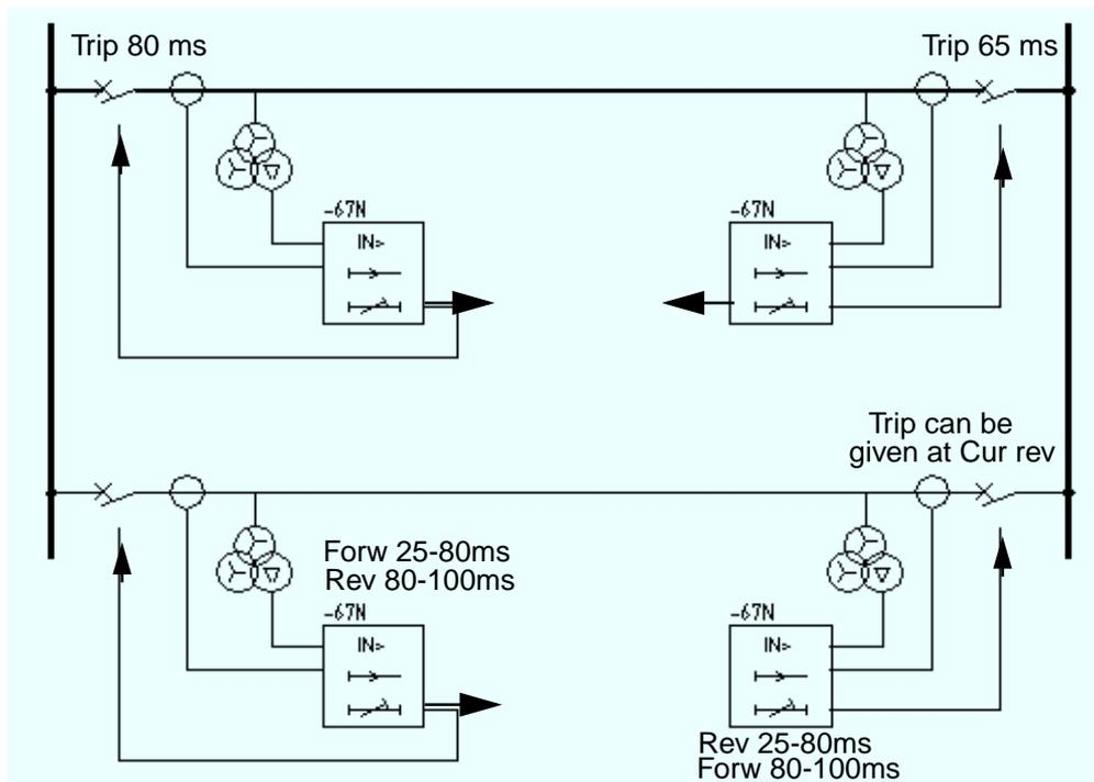
Figure 9. The current reversal problem at parallel lines.
