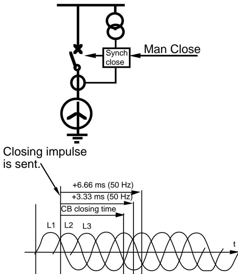
Figure 2. Synchronized closing of Shunt Reactor Circuit Breakers.
