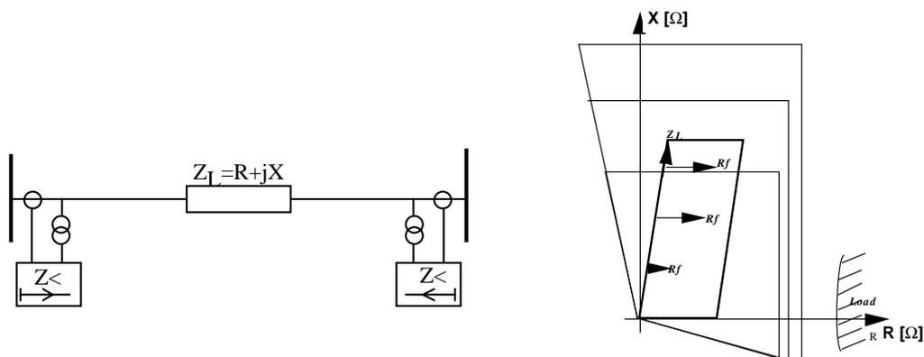
Figure 7. The principle of a Distance protection relay.
