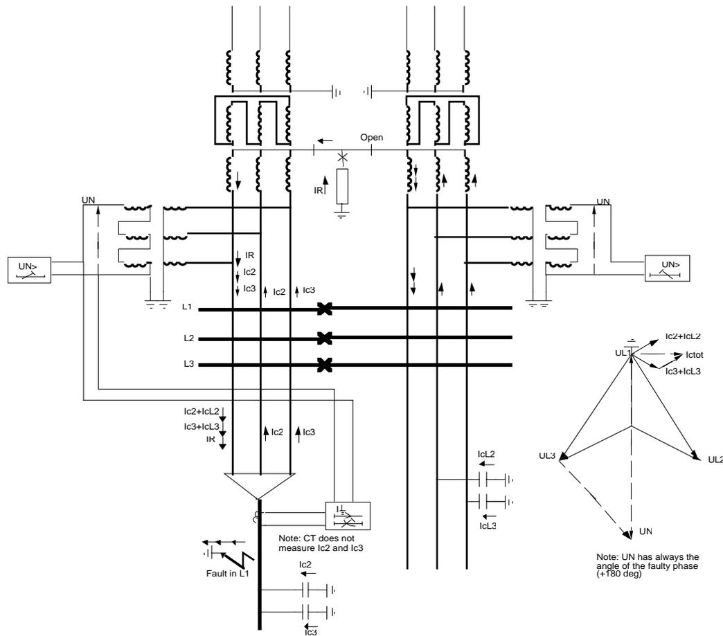
Figure 15. The fault and capacitive current distribution in a high resistance earthed network.
