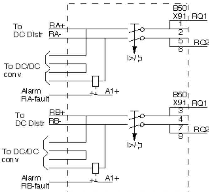
Figure 8. Supervision of the DC supply to a protection panel, detecting faulty supply fuse, open circuit and DC/DC converter failures.
