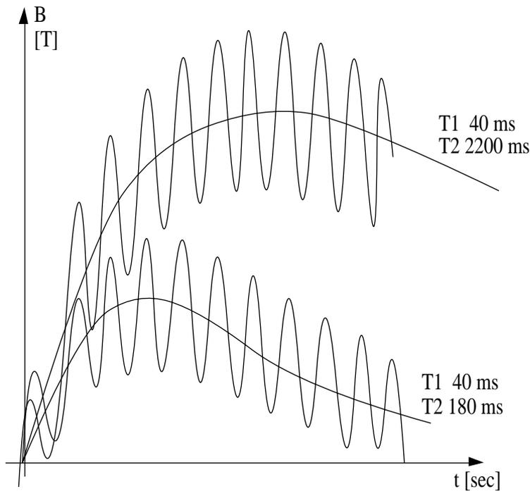
Figure 3. AC and DC flux dependent of time, at faults with full DC component and with different primary and secondary time constants.
