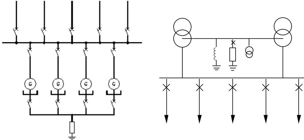
Figure 11. Resistance earthing, of the generator neutral-point, with a neutral busbar and individual neutral-point breakers.
