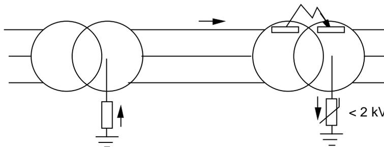
*Figure 14. Earthing with a voltage dependent resistor, to limit the overvoltage, at a break-down of a high voltage network.*
