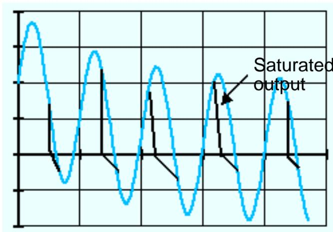
Figure 6. Secondary current at DC saturation. For some cycles the positive part of the sine wave will be destroyed.
