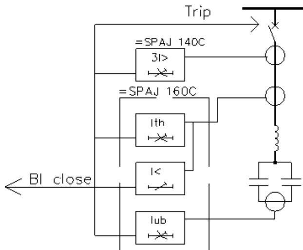
Figure 2. A SPAJ 160 connected to a capacitor bank.
