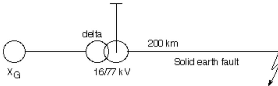
The line is considered unloaded before the fault and all resistance and capacitance is neglected. The voltage at the fault position is 75 kV before the fault.
