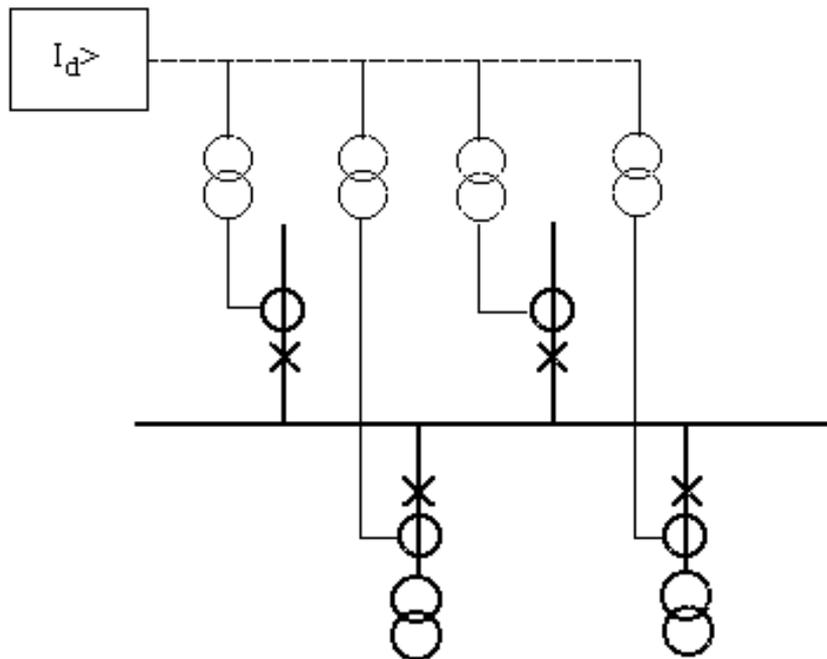
Figure 1. A one zone differential relay for a single busbar.
