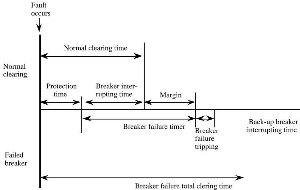
Figure 8. Time scheme for breaker failure relays
