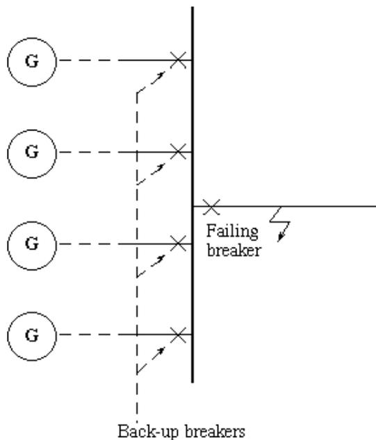
Figure 7. The principle of a breaker failure protection.
