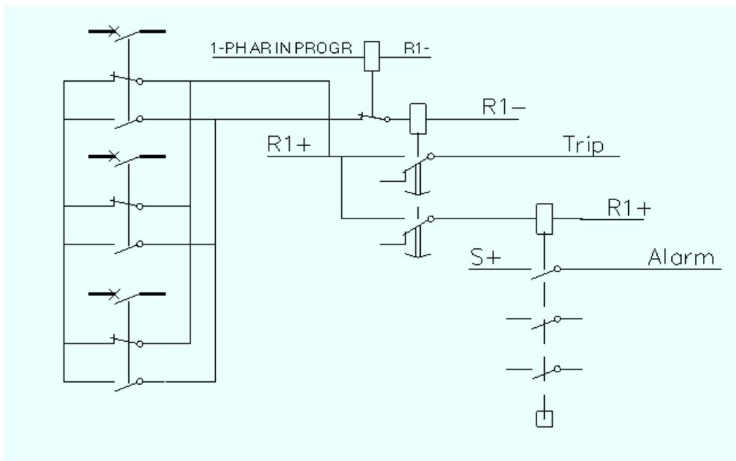
Figure 9. Connection of a Pole Discordance relay.
