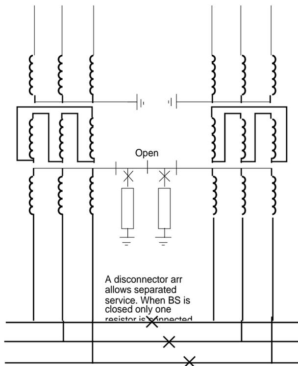
Figure 14. A high resistance earthed network and a selection of service conditions with disconnectors.
