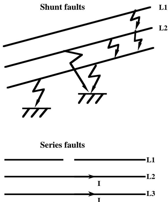
Figure 2. Different fault types in a power system.
