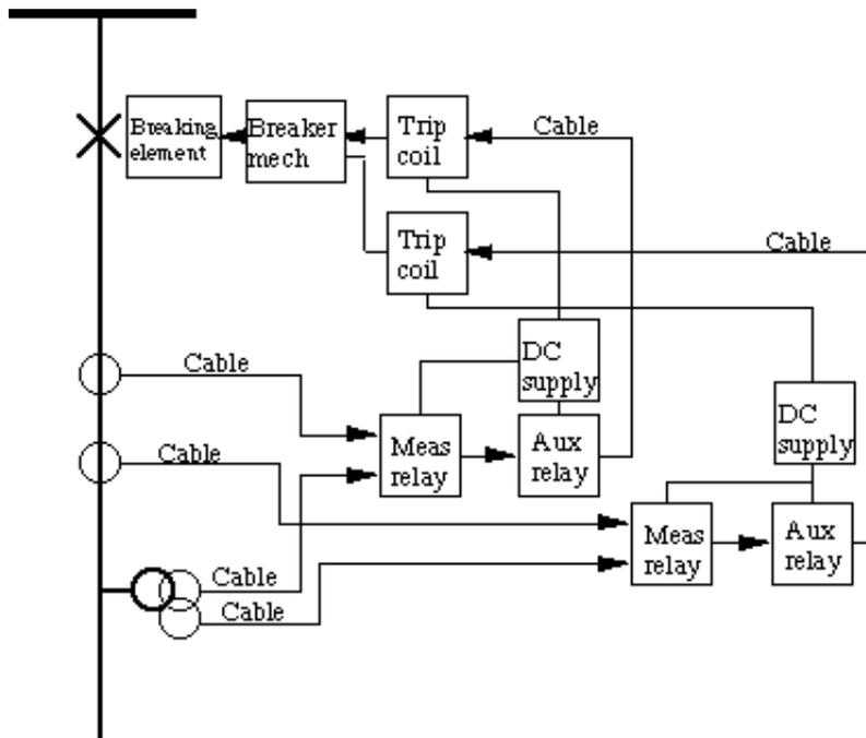
Figure 2. Fault clearance chain at redundant protection systems
