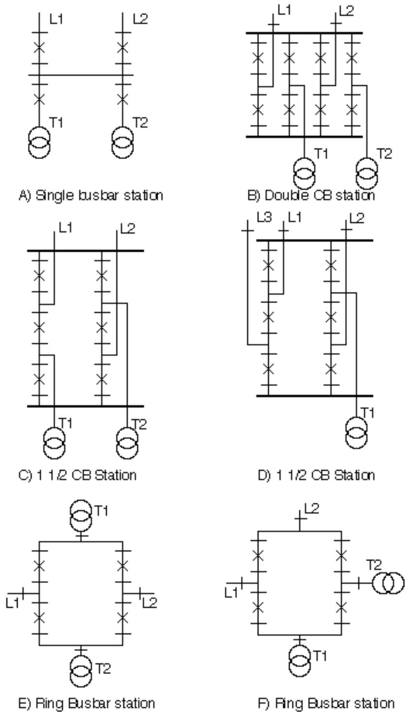
Figure 25. Examples of multi breaker switchgear arrangements
