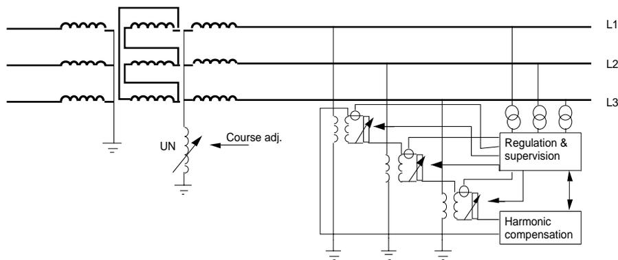
Figure 18. A compensation equipment for neutral point unsymmetry.
