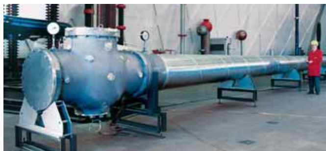
Fig. 2.5-4: Siemens lab prototype for dielectric tests
