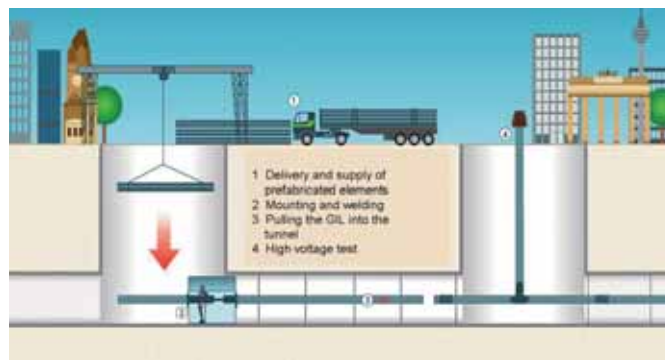
Fig. 2.5-3: GIL laying technique
