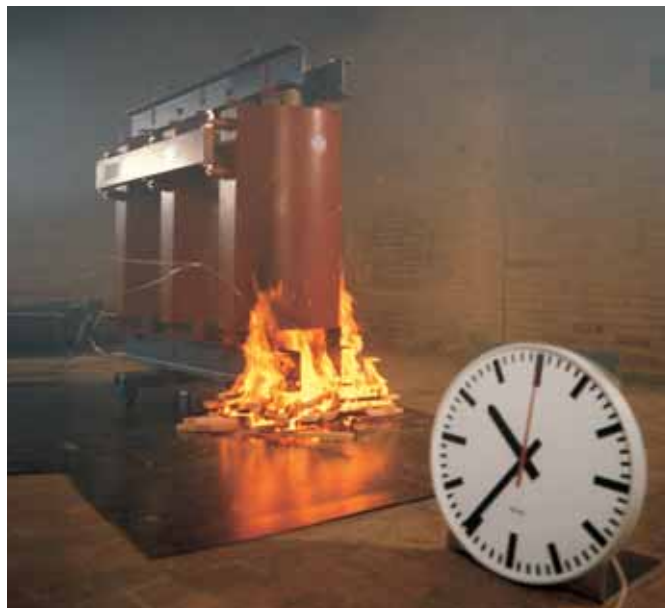
Fig. 5.9-6: Flammability test of cast-resin transformer
