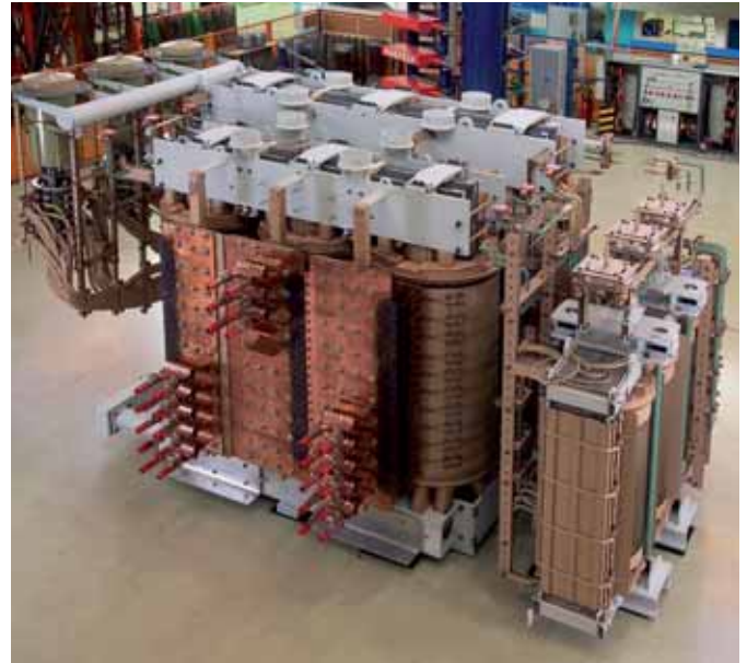
Fig. 5.6-2: Active part of an electric arc furnace series reactor
