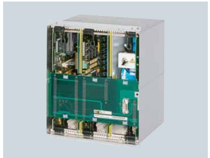
Fig. 6.4-16: SIMEAS R, front view – a DAU can be seen in the middle slot
