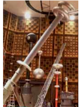
Fig. 2.2-4: UHV DC bushing at the test lab
