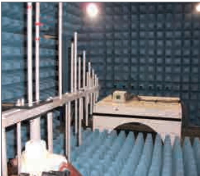
Figure E1.14: Example of radiated test immunity in semi-anechoic chamber
