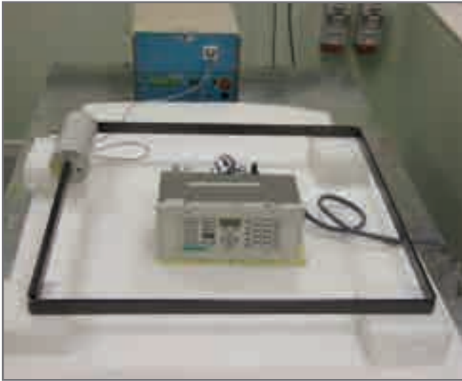
Figure E1.15: Example of power frequency/pulse/damped oscillatory magnetic field test equipment
