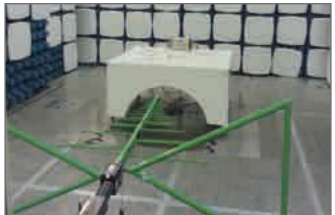
Figure E1.12: Example of radiated emission test equipment
