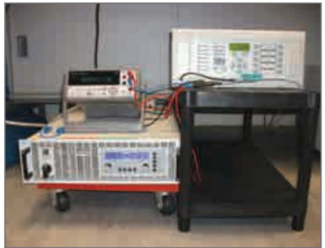
Figure E 1.18: Example of earth bonding impedance test done between the front panel of the protection relay and the metal parts
