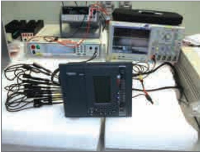
Figure E1.16: Example of set-up of dielectric test with generator
